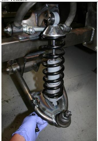
Once the lower shock bolt is tight you can now lift the control arm up into place and install the upper shock bolt.
